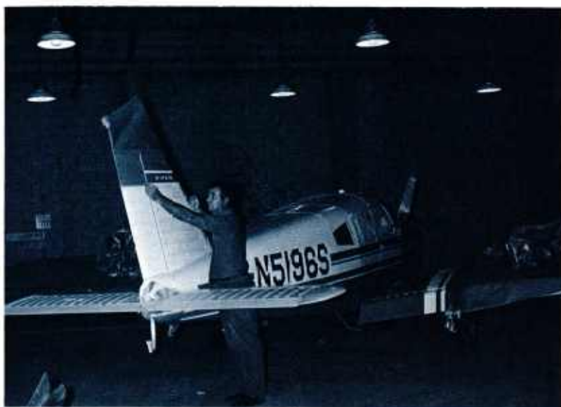
FIGURE 107 Masking trim; painting
